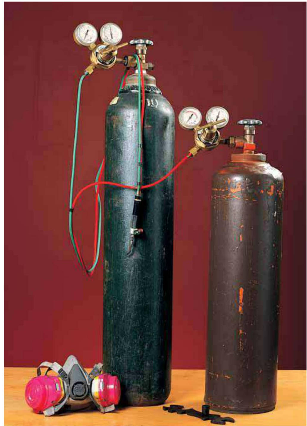
The oxy/acetylene system is comprised of two tanks, each with regulators: oxygen and acetylene, connected to the torch with the proper connecting hoses; a tank wrench and a respirator are also necessary.
