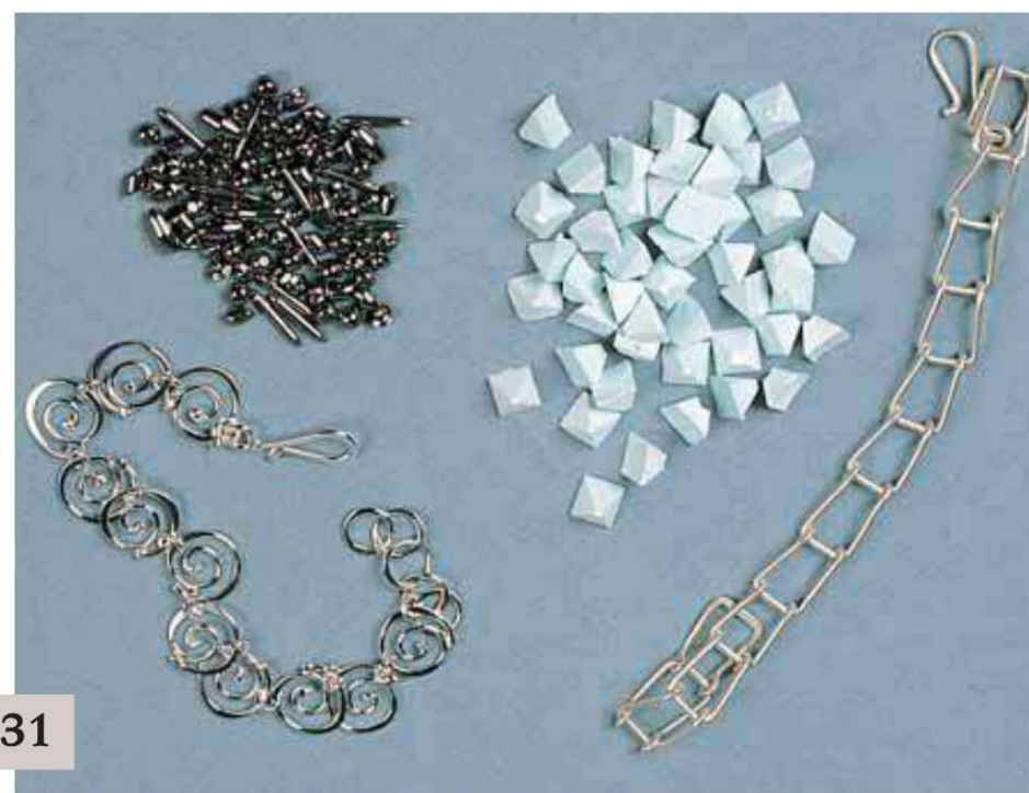
A high polish finish is created by stainless steel shot, and ceramic media produces a satin finish.
