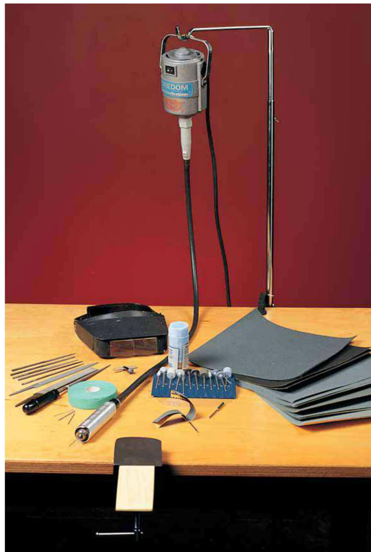
The polishing station needs (clockwise from top) a flexible shaft motor (hanging from a shaft hanger); sandpapers; a sandpaper mandrel (two are shown); a wooden bench pin (affixed in a vice to the edge of the table); a flexible shaft hand piece; self-adhesive bandage tape; various drill bits, hand files, and needle files; a magnifying visor; the hand piece's chuck key; metal lubricant; and a set of polishing wheels.
