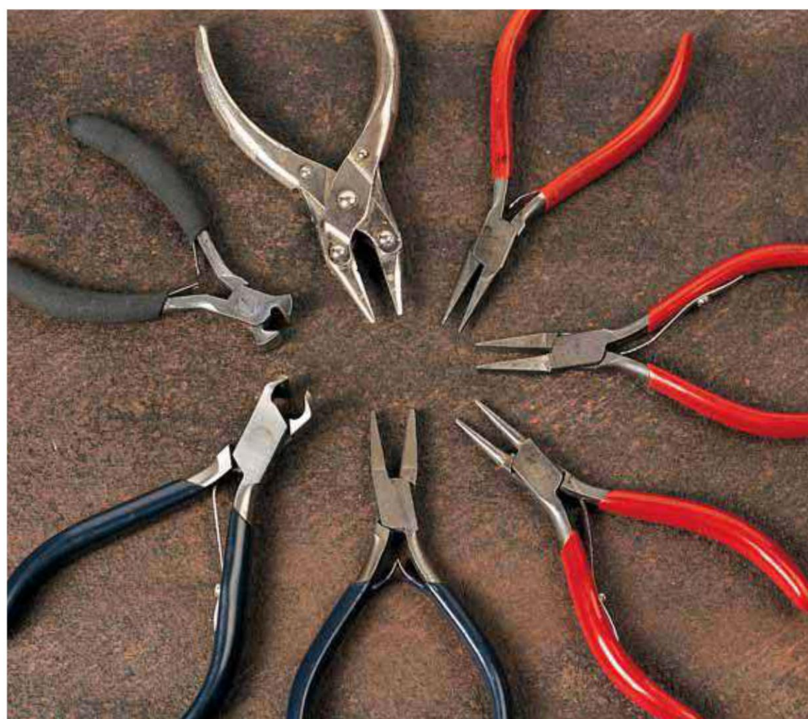
The basic hand tools (from clockwise top): box joint chain nose, lap joint chain nose, flat nose, round nose, half-round nose, large end cutters, and small end cutters
