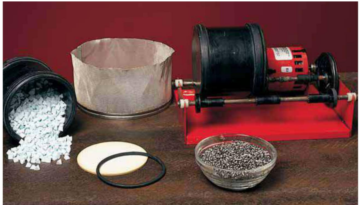
Essentials at the polishing station (clockwise from top): mesh basket, rotary tumbler with barrel, stainless steel shot, and ceramic media in a barrel, with its lid and gasket nearby
