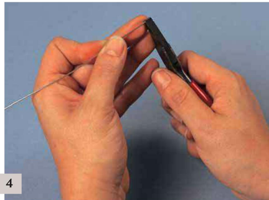
Straightening a wire by pulling against the curved tension
