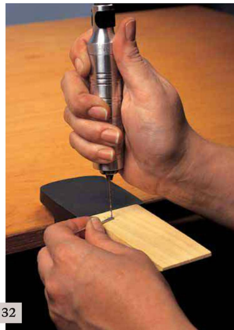
Hold the drill bit straight and square to the silver's surface.
