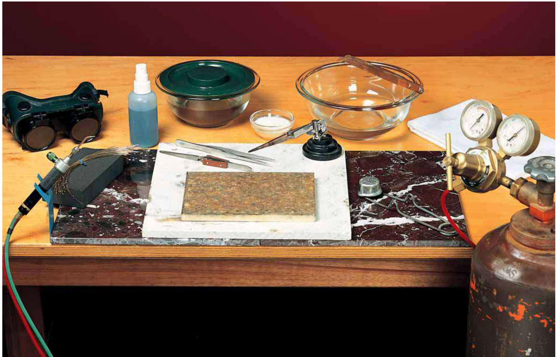
Tools for soldering include (clockwise from top) a bowl with a lid for pickle, dry pickle, a clean-water rinse bowl, copper tongs, clean towels, a fuel tank and regulator, a large stone tile, a spark lighter, soldering pad, soldering block, third hand (with black base), tweezers (two styles shown), charcoal block, wire solder, torch in a stand, shaded goggles, and liquid flux in a spray bottle.
