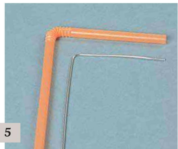
The stretched-and-crunched parts of a bend in a drinking straw are similar to the kinds of molecular changes that occur in the bent area of a piece of wire.
