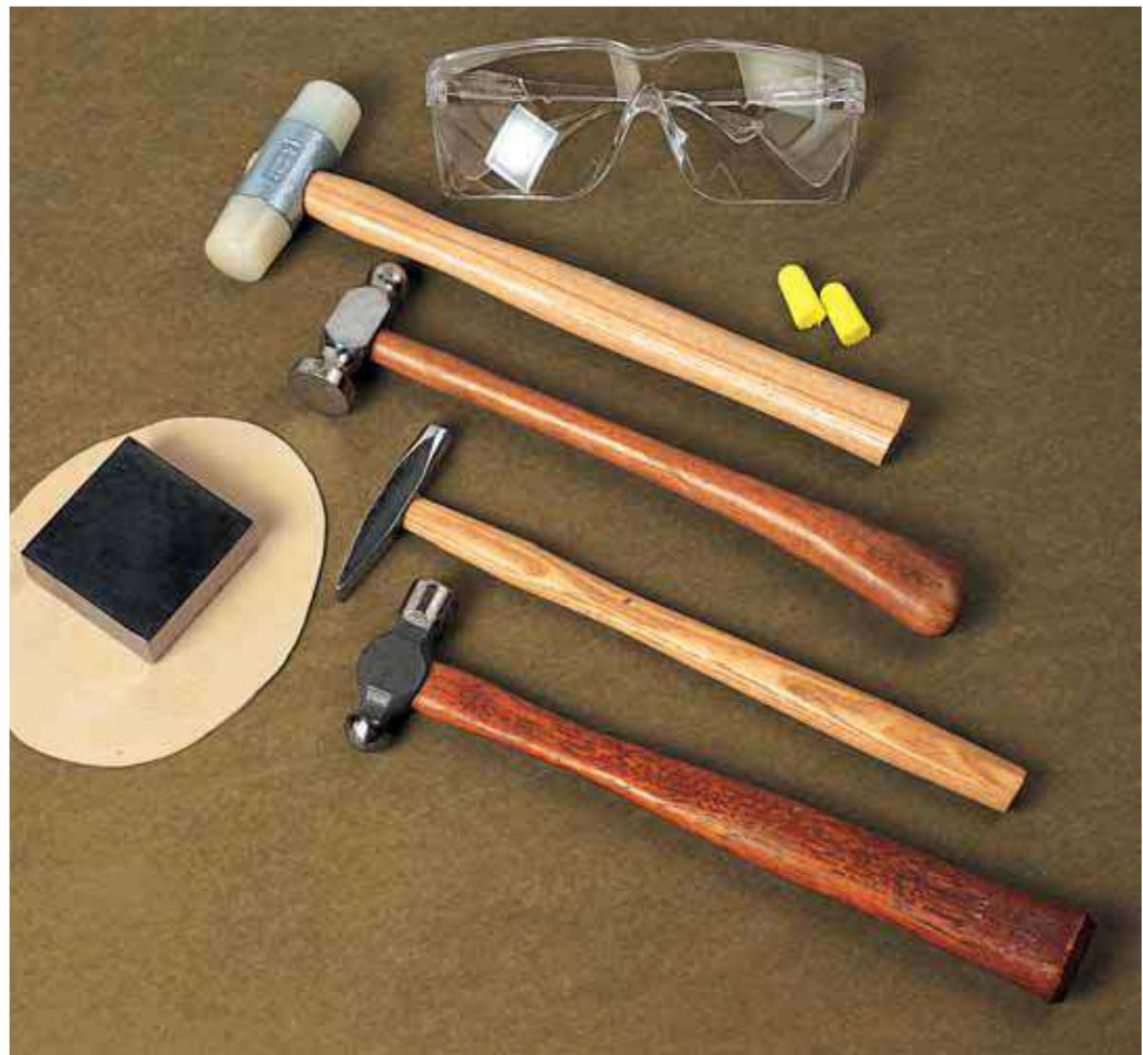
Forging tools and accessories (clockwise from top): safety glasses, earplugs, nylon hammer, planishing hammer, riveting hammer, ball peen hammer, and a bench block set on a thin rubber mat
